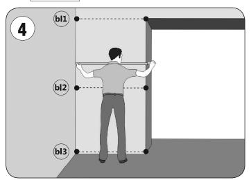
Measure the left wall (bl) to the nearest obstacle (pipe, box, wall, etc.). Write down the minimum value.
