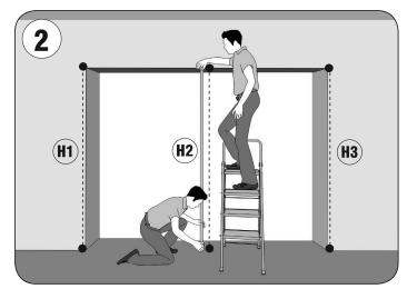
Measure the opening height (H) from clean floor. For proper measurement make sure that measurment tame on same possition. Record the maximum value.
