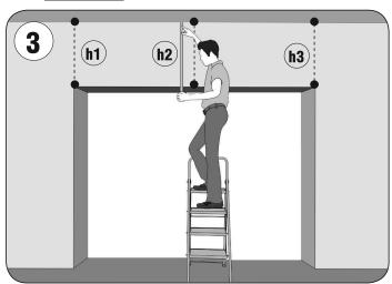
Measure the headroom of the opening (h). If beams, cables, ventilation ducts pass in the area of the headroom please write a note on the first page.
