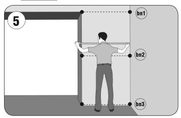
Measure the left wall (br) to the nearest obstacle (pipe, box, wall, etc.). Write down the minimum value.
